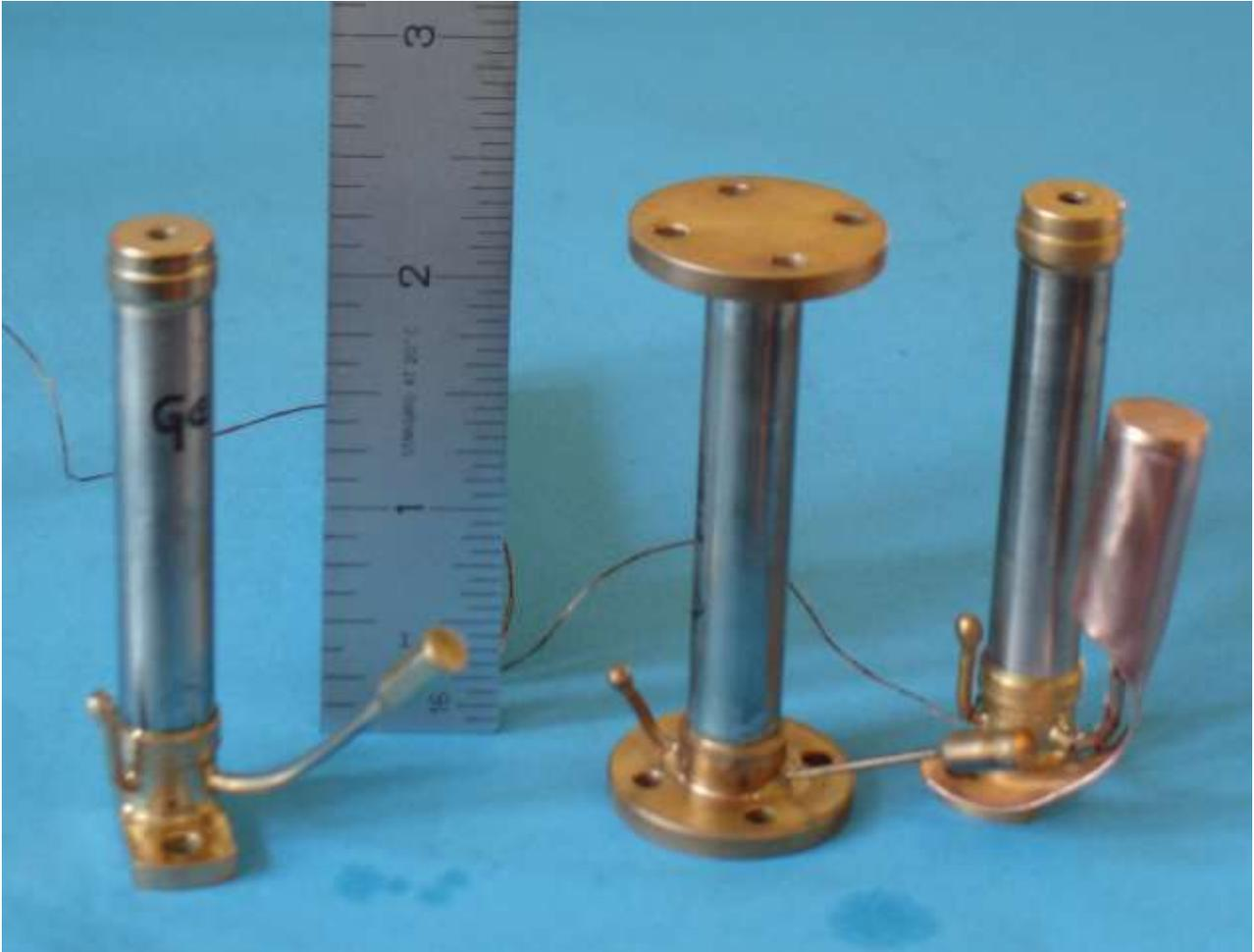
**These devices are delicate and care must be taken not to bend, twist or drop them. Distortion is likely to cause a thermal short.**
