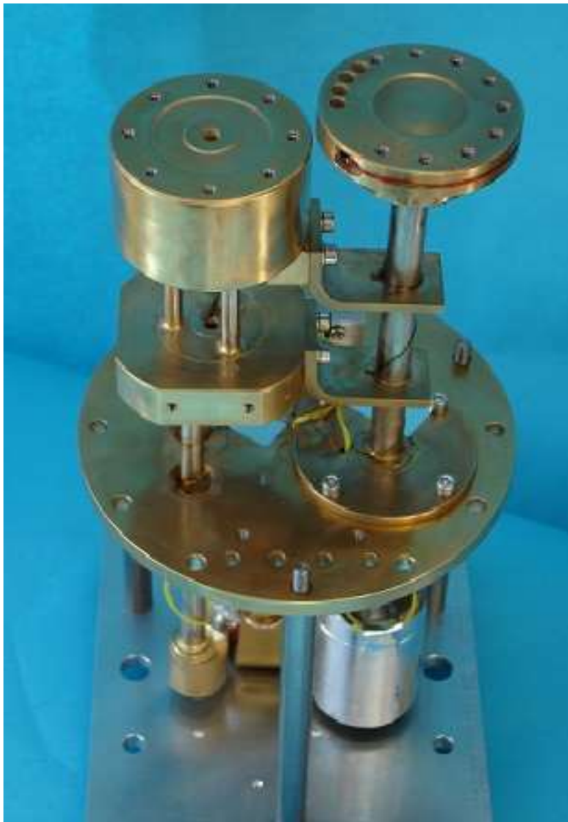
Photo shows a typical CRC GL7 (Helium 7) cryocooler
